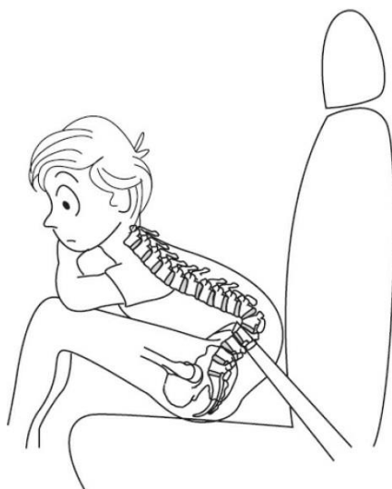
Figure 21-1. A lap belt used for a child can create a point of rotation about which the spine is flexed with an abrupt stop. This is a common mechanism for creating both intra-abdominal and flexion-distraction spinal injuries.
